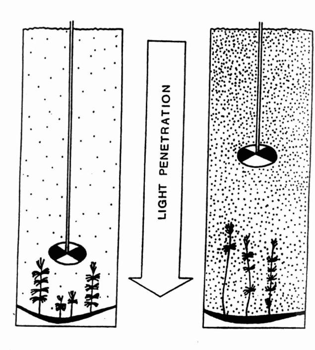
Figure 1: Diagram illustrating the use of a Secchi disc to measure water quality. Good visibility characterizes clear lakes with low algal densities (left panel). Poor visibility characterizes productive lakes with high algal densities (right panel).
